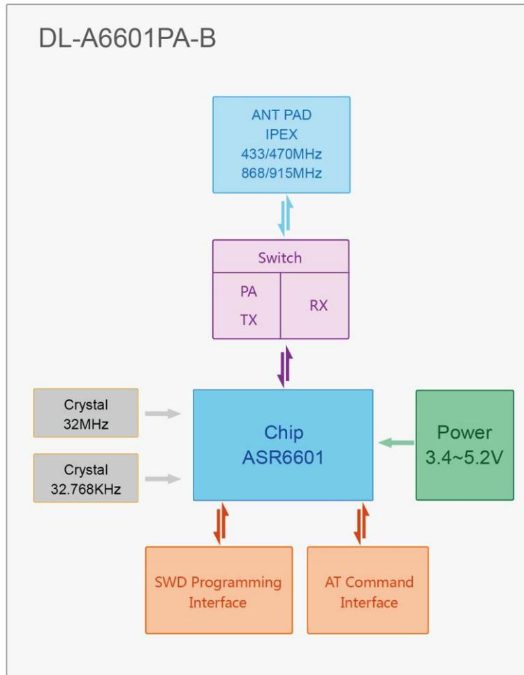
Circuit Schematic Diagram (DL-A6601PA-B)
